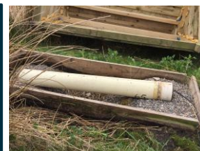
Fig 1C. [top] An induction coil magnetometer at ESK oriented in the X-Y direction.
